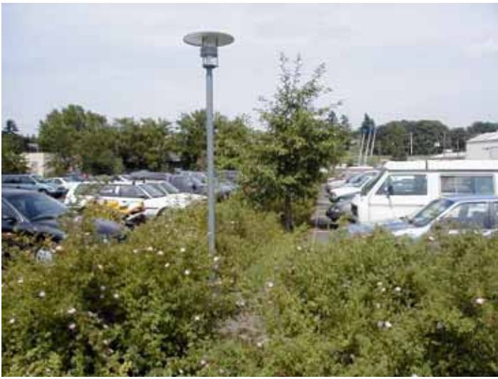
Figure 6. Bioretention practices used to accept and treat stormwater from parking areas in Portland, Oregon (left) and Evergreen Walk Mall in Manchester, CT (Right).
