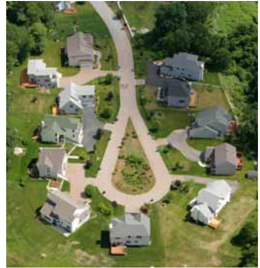
Figure 2. The “tear drop” cul-de-sac design used in the Glen Brook Green Subdivision
